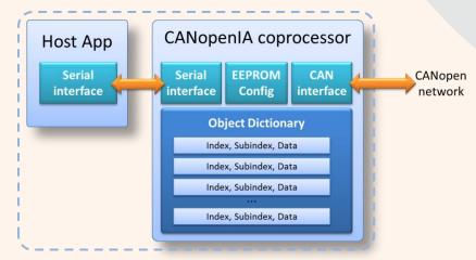
Use ESAcademy's CANopen Architect software to start a new configuration or import an existing one, for example an EDS (Electronic Data Sheet) or CODB (CANopen data base) file. Once the desired configuration is finished, save it as EDS or binary EDS. Then, transfer the binary EDS configuration to a CANopenIA implementation using any CANopen
