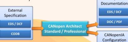
Use the CANopen Architect software to start a new configuration or import an existing one, for example an EDS (Electronic Data Sheet) or CODB (CANopen data base) file. Once the desired configuration is finished, it can be exported and loaded into CANopenIA devices.
